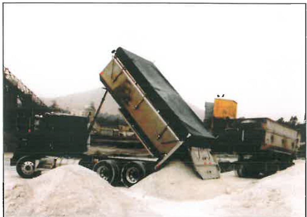
Truck body recently built in DTI's Adelanto Shop. Note the form-fitting tarp for dust control.
