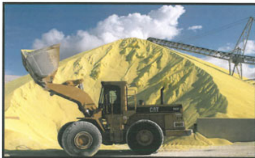
To speed loading, two loaders are used. One loader places three scoops in the front (semi) trailer and while the second places two scoops in the rear (pull) trailer. Payloads are approximately 24.5 metric tons.
