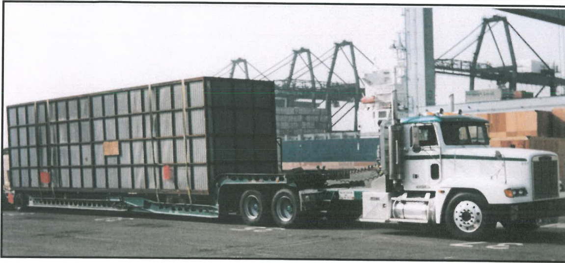
Left is a 40' imported machine in Long Beach makes good use of one of our deck extensions. Note the container is slightly longer than the 34' now in the well.
