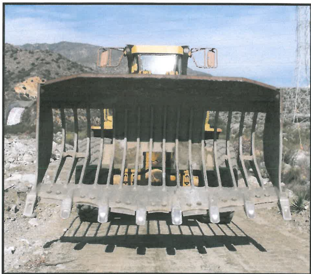
Above, Front View of the skeleton bucket to sort out finer material from desired sizes. Below, Partial view of Dalton's boulder inventory stored in Fontana for easy sorting, loading and delivery.
