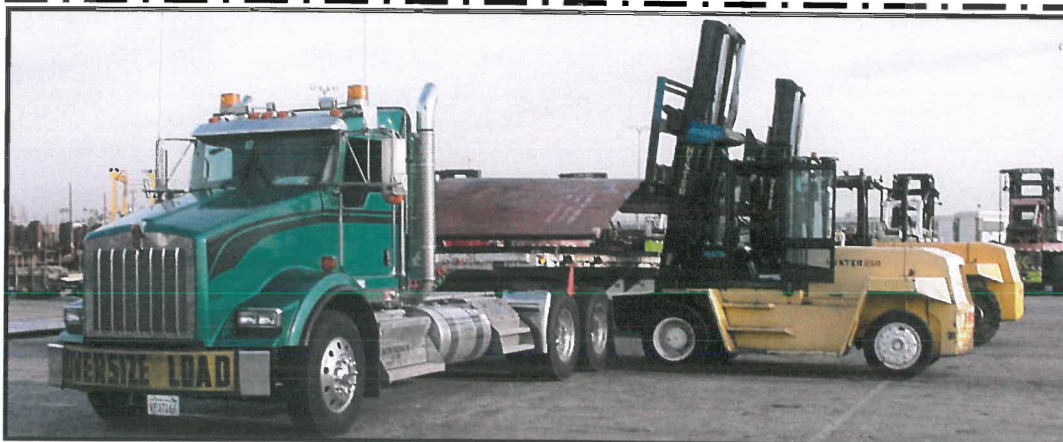
Above is a pair of 30,000 lb forklifts loading 40' long plates onto one of Dalton's CARB compliant 2008 tractors.
