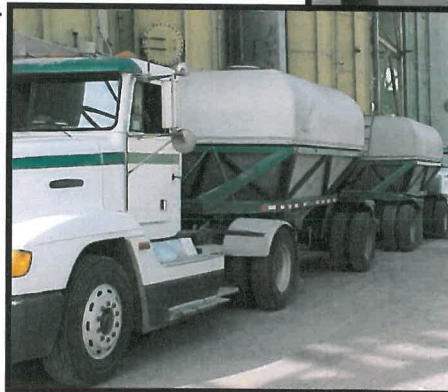
Pictured left is a set of Dalton's covered dome hopper trailers, setting in place to unload product into a grizzly. Top, the granular bulk commodities are gravity unloaded into a grizzly. Note the canvas boot used to reduce dust.
