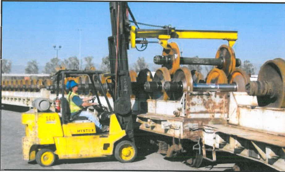
One of two hydraulic ram attachments for our forklifts handle a newly refurbished axle/wheel set for reloading.
