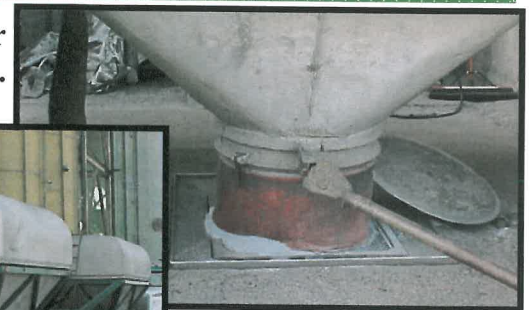
Pictured left is a set of Dalton's covered dome hopper trailers, setting in place to unload product into a grizzly. Top, the granular bulk commodities are gravity unloaded into a grizzly. Note the canvas boot used to reduce dust.
