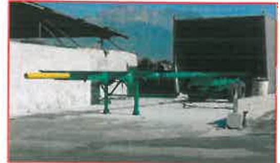
Almost finished after sand blasting and paint. Wiring and tires were all that remained.
