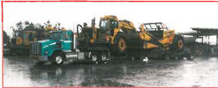
This rear view of the three Cat 657's shows their rear engine assembly and hence the need for the third booster axle to handle the added weight.
