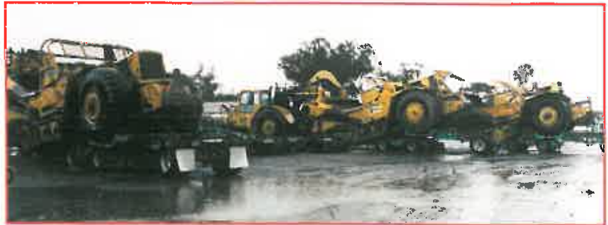
This rear view of the three Cat 657's shows their rear engine assembly and hence the need for the third booster axle to handle the added weight.
