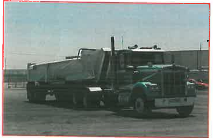
After the brick was run through DTI's grizzly to sort the material, it was then hauled in semi-end dumps from their Riverside plant to their plant in Oro Grande.
