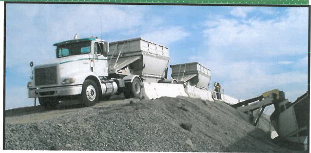
Above is one of our lightweight bottom dumps (hauling around 27 tons) pulled over a raised drive over grizzly hopper which feeds a radial stacker. This high volume system can handle over 20 trucks per hour.
