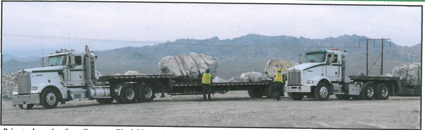
Prior to departing from Cemex at Black Mountain, these stones must be carefully placed on the trailer and because of their irregular shapes; sometimes four or five chains each must be used. Often as in this case, drivers will help each other tie down
