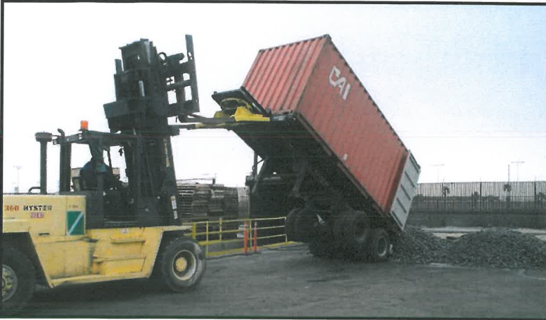
Pictured here is our 36,000 lb Hyster forklift dumping approximately 45,000 lbs of metal alloy from a sea container.
