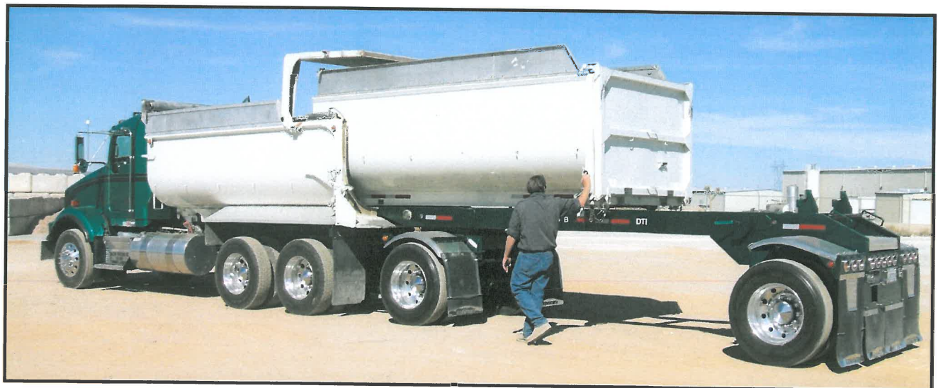
Above is one of our drivers operating the controls to place the transfer body inside the truck's dump body shell. Our transfers are just what you need for tight areas where you can't get a pup or semi trailer.
