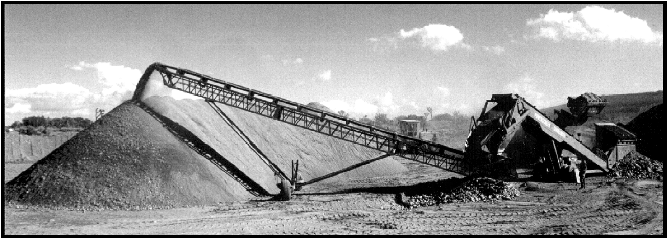
Finished product pours from radial stacker at San Bernardino County Disposal Site near Phelan, CA.
