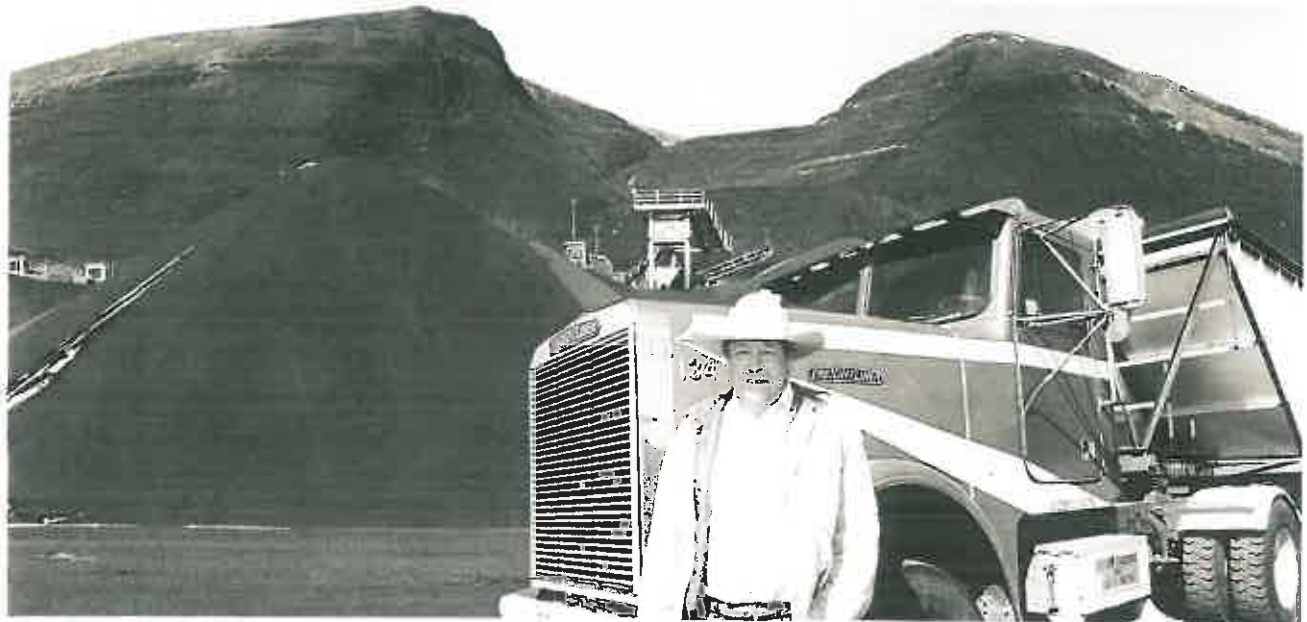
Mining cinders for snow control is mainly a winter endeavor, but cinder production for lightweight aggregate continues year-round. Don Jolly is pictured with a 50 cubic-yard bottom dump set.
